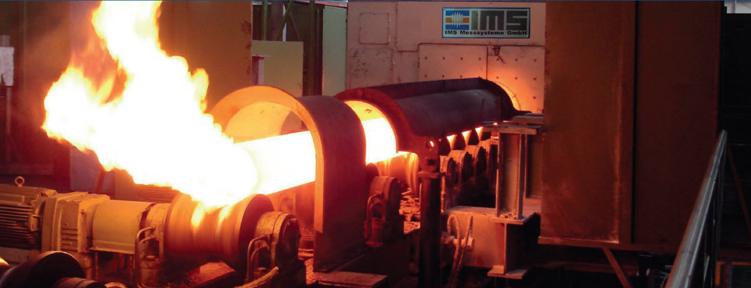
Inside view of IMS 13-Channel Tube Wall Thickness Measuring Gauge
